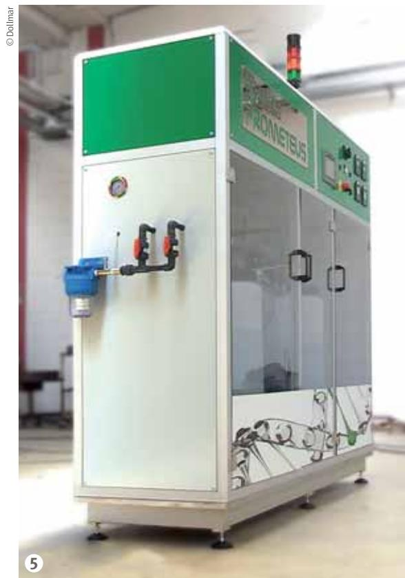
**Figure 5: The PROMETEUS nebulisation module for the nanotechnology conversion process.**
