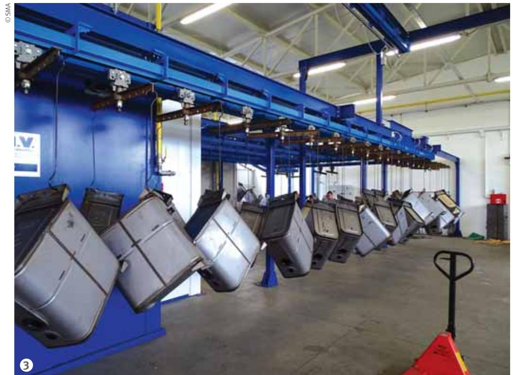
Figure 3: Tanks waiting to enter the pre-treatment tunnel.
